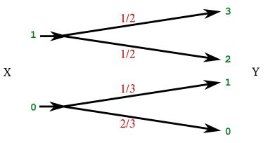
Channel appears to be noisy, but really isn't, as we can exactly determine the input from the output.
