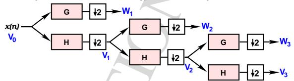
Each block refers to the use of one of the filters defined above followed by a downsampling, and each filtering corresponds to a convolution, for instance, the two first filters result in
