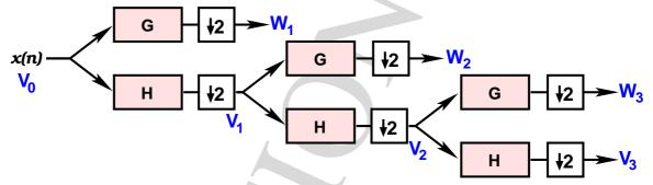
Each block refers to the use of one of the filters defined above followed by a downsampling, and each filtering corresponds to a convolution, for instance, the two first filters result in
