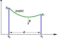
Catenary problem where we have pullies on top of each pylon, and a large amount of cable. Under appropriate conditions it will reach an equilibrium shape. The critical features of this problem are that the end-points are fixed but the length L of the cable is unconstrained.
