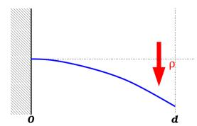
But this can fail in some cases, for instance, if the left end of the cantilever isn't clamped (to have zero slope) then the right end can swing freely, and  $x_1$  won't be fixed.
