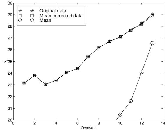
(b) The Logscale Diagrams of the original data (\*), the corrected data ( $\square$ ), and the fitted transition function ( $\circ$ ).
