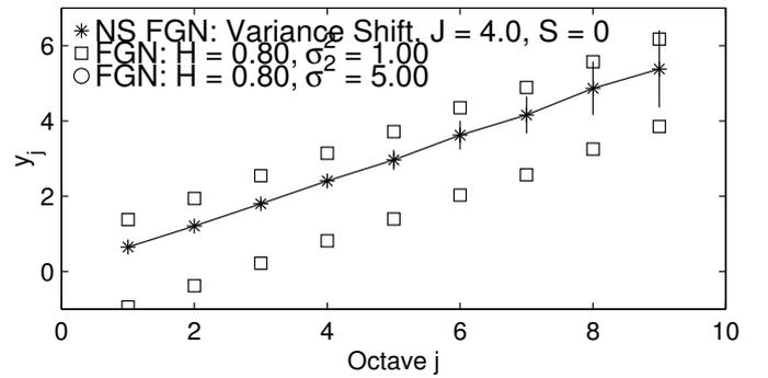
Fig. 5. An example Logscale Diagram for a change in the variance,  $H = 0.8$ . The (\*) show the sample mean of the  $y_j$  for the NS FGN, and the ( $\square$ ) and ( $\circ$ ) show the sample mean of the  $y_j$ 's for FGN processes with variance matched to that of the NS FGN at time 0 and time  $n$  respectively. The vertical lines show the one standard deviation of the NS FGN results.
