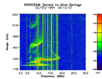
The two polarization modes appear as two superimposed copies of the F-layer traces.
